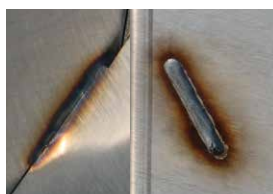
TAB WELDED HOPPER CONSTRUCTION
